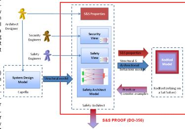
safety and security domains are quite different in terms of practices, concepts used and wording. The tool chain developed for this purpose is the following: The system architecture model is built with Cappella (Thales) and then imported into Safety Architect (All4tec) to perform Safety and Security analyses. The results are translated into Alloy so that both safety and security properties can be verified with the Kodkod Analyser (SAT solver - Onera).
